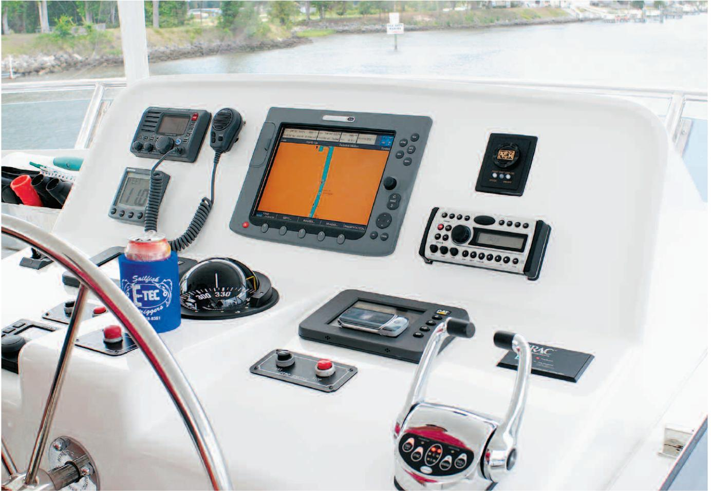
The flybridge helm features a range of owner-selected instruments and electronics, including a remote-operable shift and throttle control.
