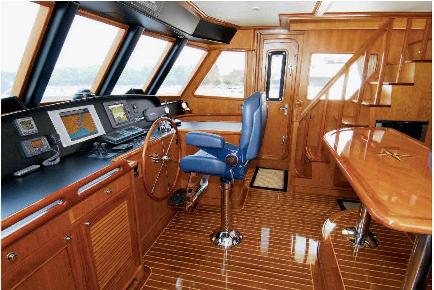
The Outer Reef's gleaming pilothouse is comfortable and user friendly. The Stidd chair, table, and settee (farther aft) provide ample accommodations for those on and off watch. Note the generously proportioned companionway to the flybridge.
