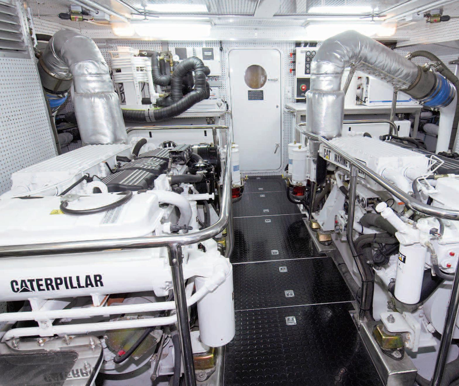
“Bright” and “clean” are the first words that come to mind when describing the engine room. Access to the twin Cat C9s, generators, and other gear is excellent. The engine room also is equipped with a fixed clean-agent fire extinguishing system.
