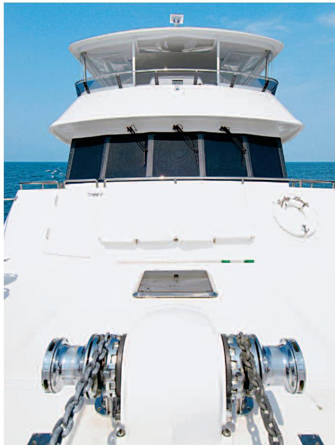
Top right: Note the intricate design of the stainless steel anchor chafe protector on *Lucky Linde*'s bow. Stainless design, fit, welding, and polish are outstanding throughout the Outer Reef 65. Above: With a big Maxwell 3500 anchor windlass and Portuguese bridge, the Outer Reef's foredeck is all business.
