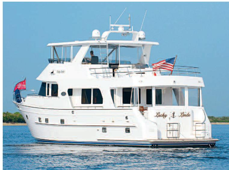
With ample rubrails and spray rails, a high freeboard, and substantial bulwarks, this vessel is ready for extended cruising.
