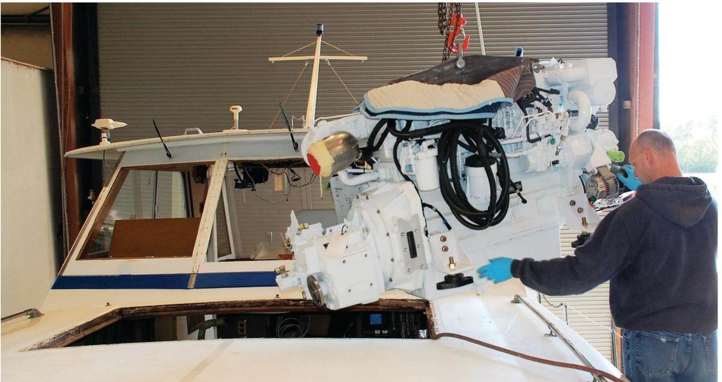
*Eventually time and wear catch up and the situation will call for a rebuild, a remanufactured engine, or, in this case, a new engine.*
