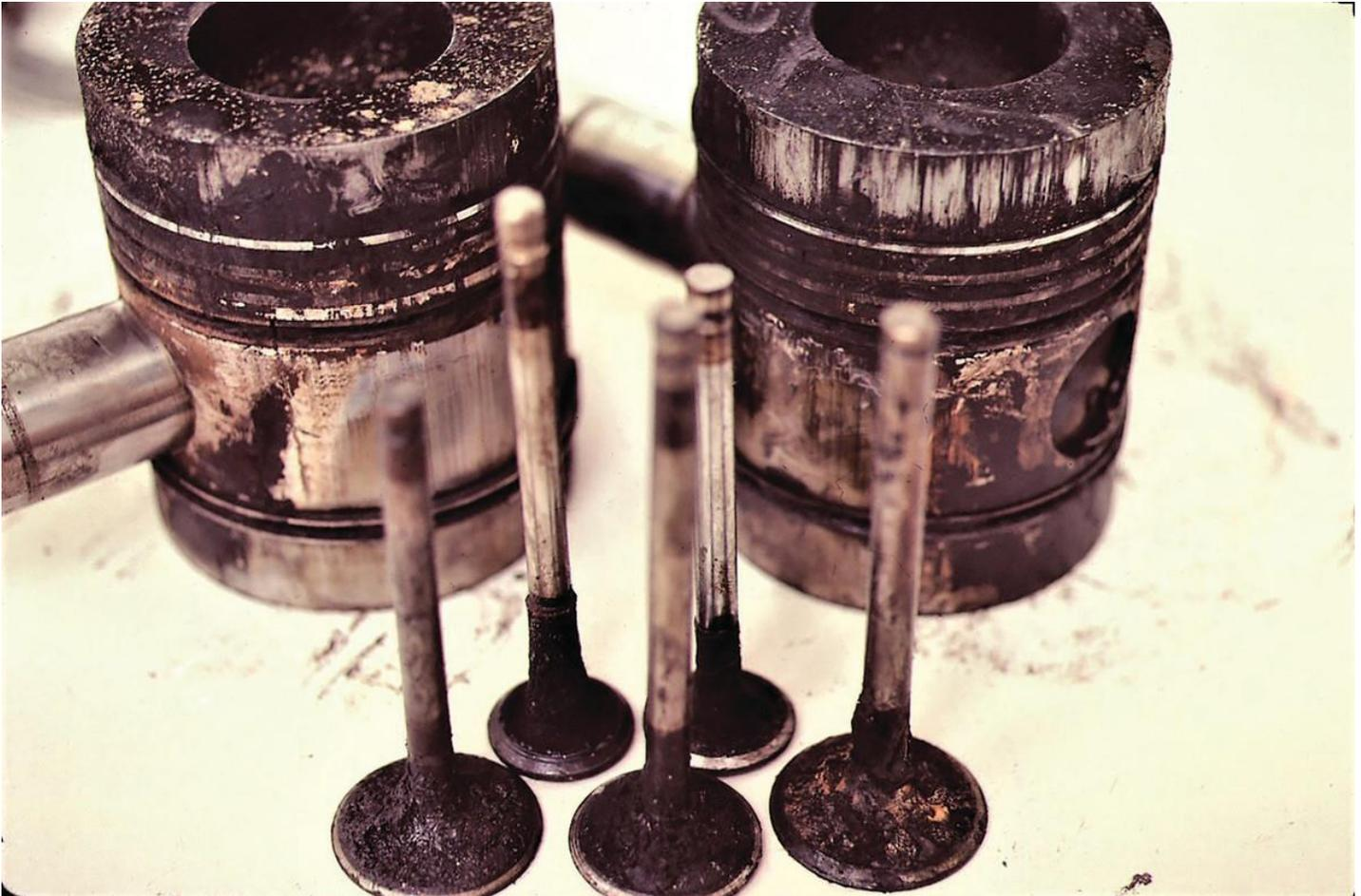
*Chronically running at light loads can lead to a build up of carbon deposits in the cylinders and exhaust components. Over time this can lead to premature engine failure. This engine required a rebuild after only 700 hours. Nigel Calder*
